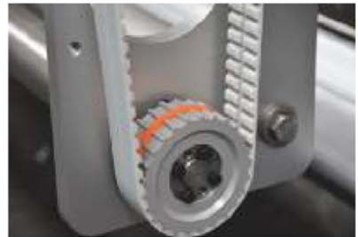
Timing belt used for robotic arms
